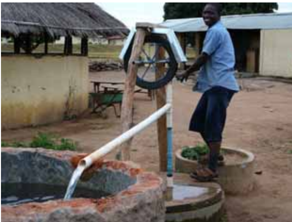
Filling the tank with the hand rope pump in Chimoio
