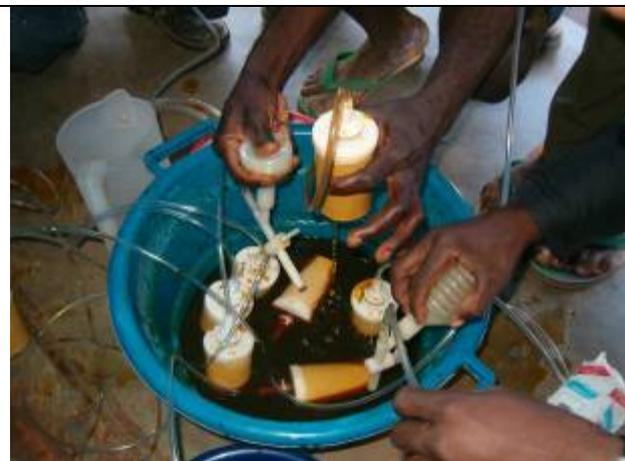
*The filters being treated in water with colloidal silver*
