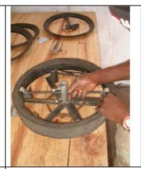
Using a Jig to weld the clamps and spars to the Hub. The spars should fit tightly.
