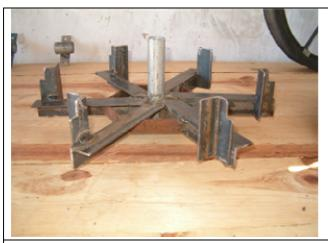
Jig for proper assembling of the wheel.
