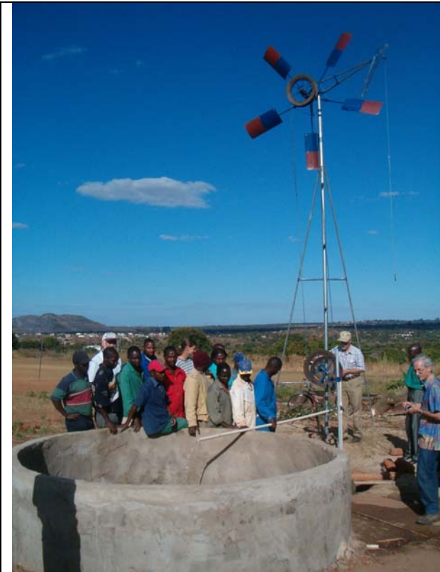
First wind rope pump built and installed in Chimoio Mozambique, 4 th of June 2006, with 6.5 cub m water tank
