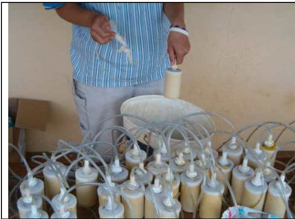
Preparing the stefani ceramic filters with colloidal silver solution, Chimoio
