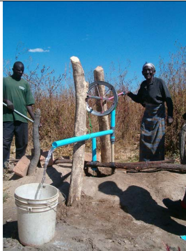
First hand rope pump installed for old lady near Childrens Town , Chibombo, Zambia
