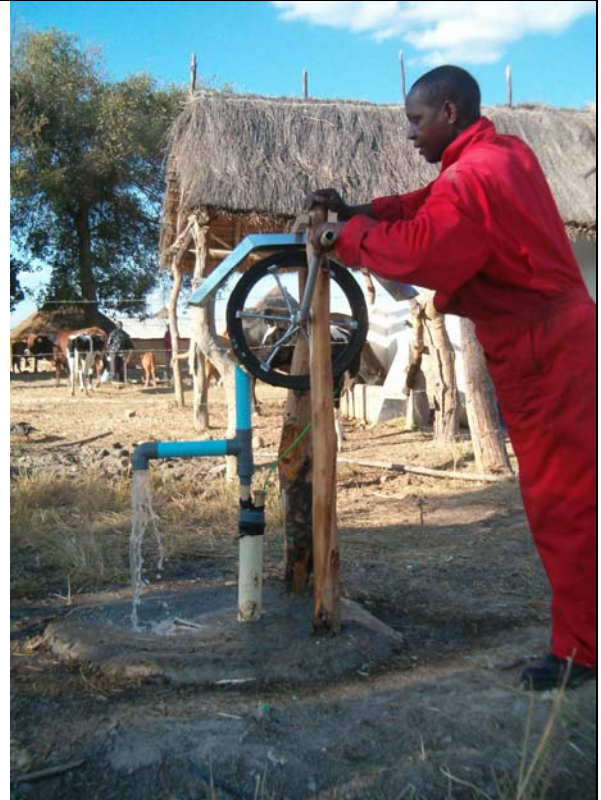
Hand rope pump at 75 mm borehole in Chibombo
