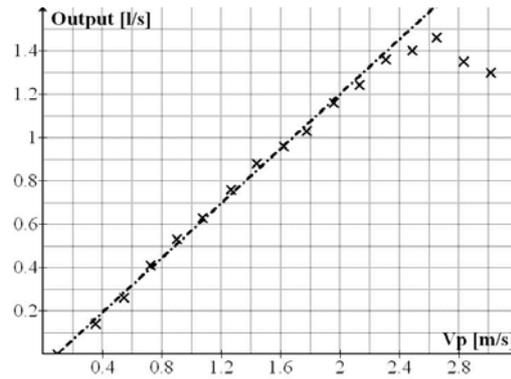
Figure 7: Flow measurements carried out by Gómez [16] for a rope pump with a diameter of 1", showing the linear relation between the output and the rope speed upto 2 m/s. The piston spacing ( $1/N$ ) was 1.04 m. The existence of a critical rope speed  $V_c$  is clearly visible, as well as the effect of increased losses at higher rope speeds.
