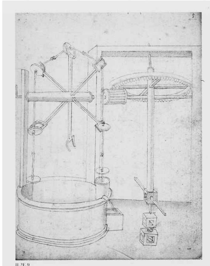
Figure 1: *The pump depicted in the left part of this anonymous drawing is a chain pump (after Francesco di Giorgio). It is equipped with a chain instead of a rope but its operating principle is identical to that of the rope pump. The pump shown is driven by animal power [2].*
