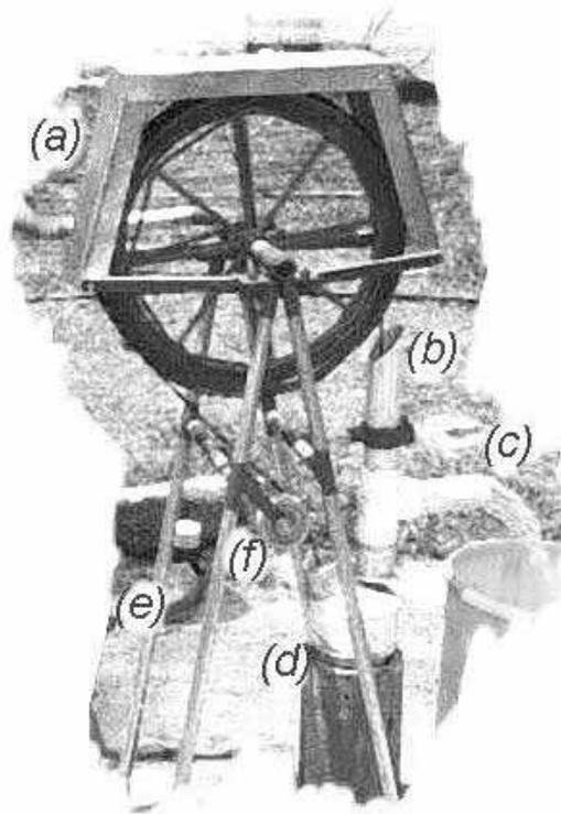
Figure 2: *Typical above-ground assembly of a Nicaraguan rope pump above a borehole, showing the following components: (a) the pump wheel with safety casing; (b) the pump pipe (rising main); (c) the discharge tube; (d) the borehole cylinder; (e) support structure; (f) pulley for rope guidance (not used on a wider dug well). The diameter of the pump wheel is 0.4-0.5 m. Behind the wheel the crank can be discerned, with which the pump wheel is turned by hand.*
