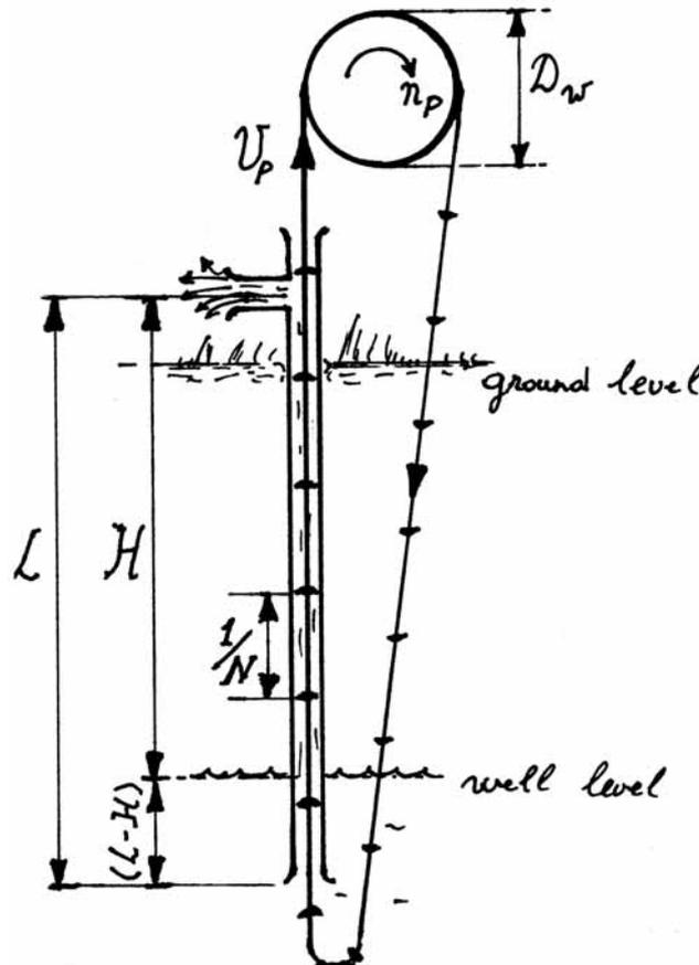
Figure 3: Basic dimensions of the rope pump: The pipe length is  $L$  and the effective pumping head  $H$ . The number of pistons per unit rope length is  $N$  and the diameter of the pump wheel is  $D_w$ .
