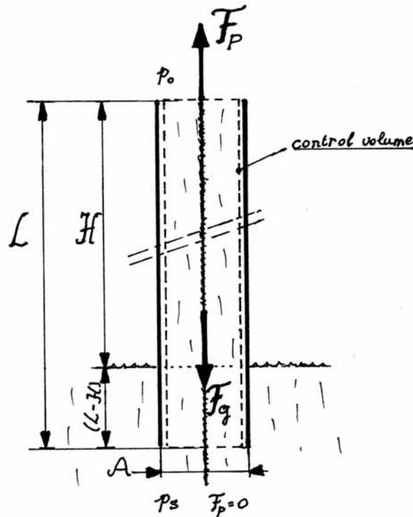
Figure 4: Balance of the rope force  $F_p$ , gravity force  $F_g$ , and the static pressure  $p_s$  over the full pipe length  $L$  of the rope pump, applying a control volume along the inner pipe wall.  $A$  is the internal pipe area and  $H$  the overall pumping head. The pistons are not shown in this sketch.
