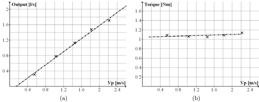
Figure 8: Measurements of (a) the output flow rate; and (b) the pump torque obtained at Eindhoven University [21]. Due to calibration problems there is uncertainty with respect to the absolute values of the torque measurements.
