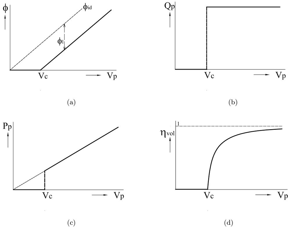
Figure 6: *Characteristic curves of the rope pump: (a) the output flow  $\phi$ ; (b) the pump torque  $Q_p$ ; (c) the input power  $P_p$ ; and (d) the volumetric efficiency  $\eta_{vol}$ . The effect of the critical pump speed  $V_c$  on the pump performance can easily be observed from these figures.*
