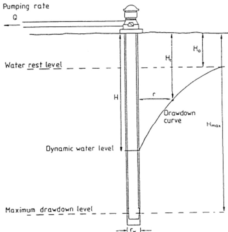
Figure 9: Water flow towards a borehole
