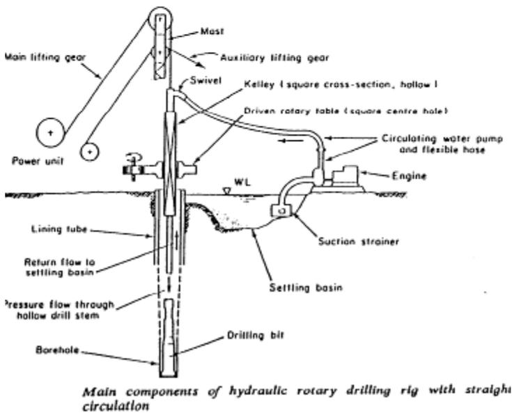
Figure 11: Drilling a borehole
