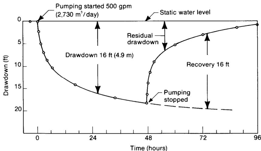
Figure 10: Typical drawdown curve for a borehole
