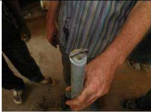
***The filter pipe made of ¾" or 1 inch pipe, closed at the top with slots made with the hacksaw***
