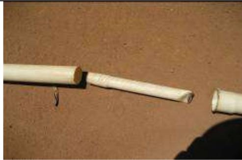
*A filter screen is made by cutting slots in an 1 inch PVC pipe and by heating and closing it at the top*
