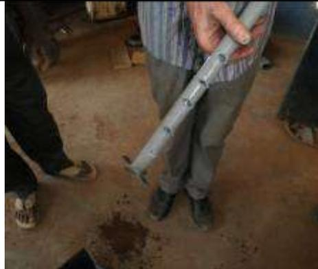
***At the lower side bigger slots and the end opened to fix the pipe in the gravel***
