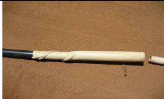
*The top of the pressure tube is made of a 1.5 Inch PVC pipe, which is heated and wound around a PVC pipe or, in this case, a black poly pipe*
