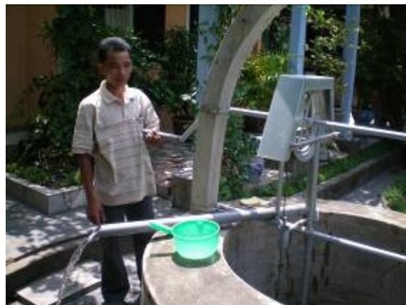
Rope pump, Windlass model in Hue
