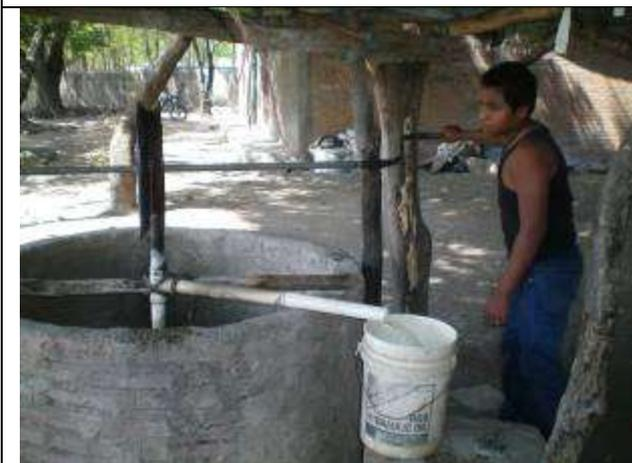
*A pole model rope pump installed in 1998. This family now has piped water but still uses the rope pump for cattle watering etc.*
