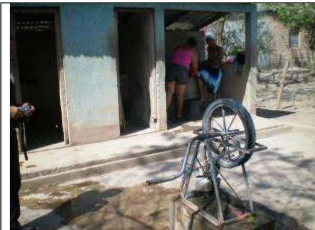
*This rope pump for communal supply was installed near San Isidro in 1998.*
