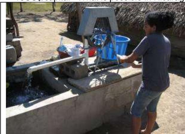
Rope pump for Self supply used for domestic use, cattle watering and garden irrigation
