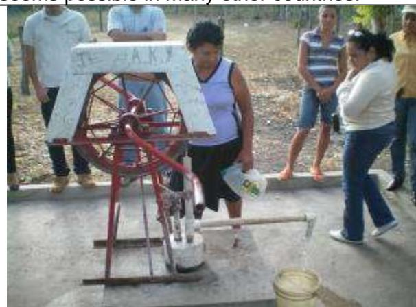
Rope pump for Communal supply on 60 mtr deep borehole of 8000US\$. Used by 20 families
