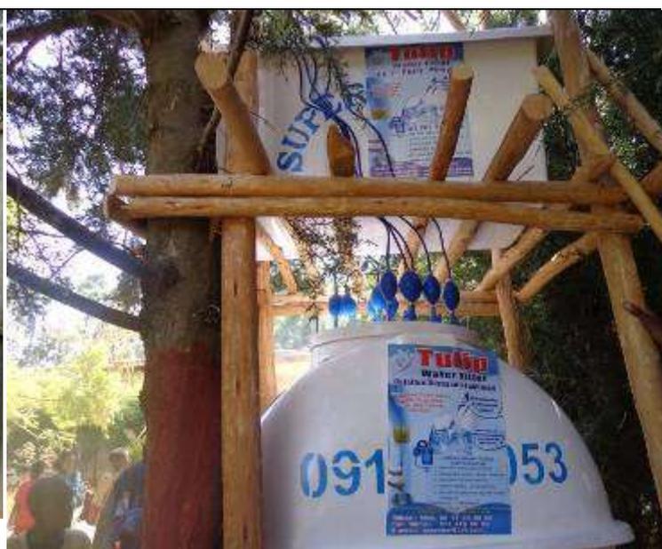
*Typical unit with upper feeding tank of 250 liter, a clean water tank of 500 liter (lower round tank) and 10 Tulip filters.
